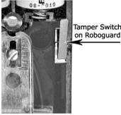
3. Press and release the Tamper Switch on your Roboguard. The Roboguard will sound 4 beeps and transmit a tamper signal, your HQ will emit 10 beeps, and all the lights will flash to indicate successful programming.
